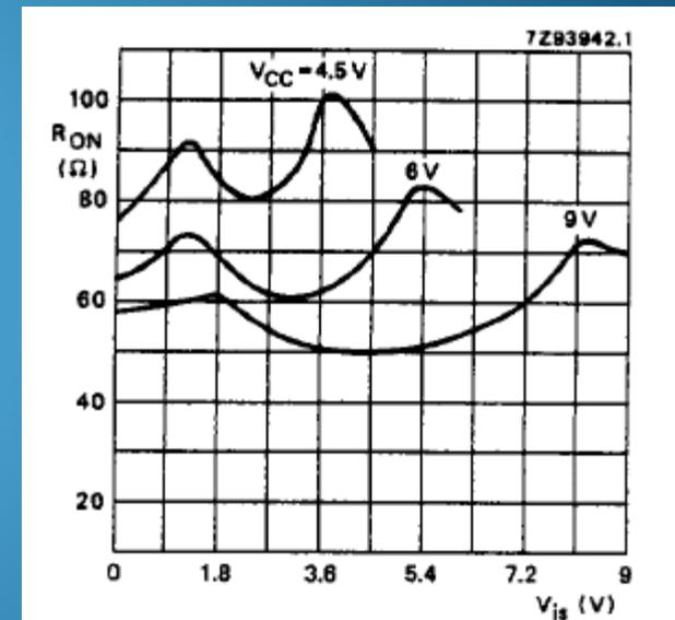
Fig.10 Typical ON-resistance ( $R_{ON}$ ) as a function of input voltage ( $V_{is}$ ) for  $V_{is} = 0$  to  $V_{CC} - GND$ .
